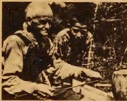
Lon smooths and trims the backs for his chairs using a drawing knife and a shaving horse. Merle, his brother's grandson, watches.
